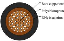
Bare copper conductor Polychloroprene rubber outer jacket EPR insulation
